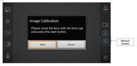
It is recommended to use the manual shutter operation just after the power is switched on or during the operation whenever nonuniformity appears.
